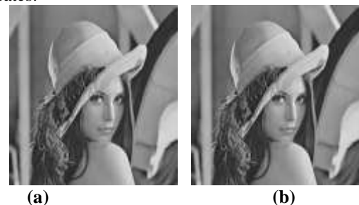
Fig.3.Reconstructed images of Lena with DTT-SPIHT at bit-rate 0.25bpp (a), (PSNR=31.5) (b) HVS on (PSNR=31.6).
