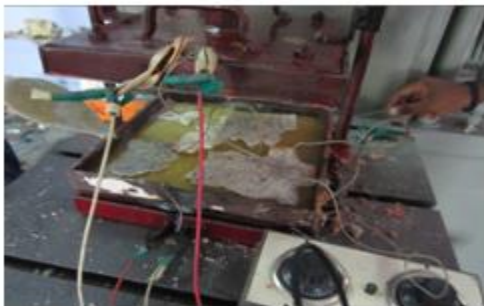
Fig.9 Compression molding Setup
