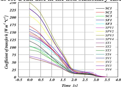
Fig. 7 Variation of heat transfer coefficient (h) of various surfaces for a ventilated disc in transient case (FG 15)
