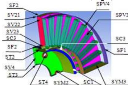
Fig 2. Definition of surfaces of the ventilated disc
