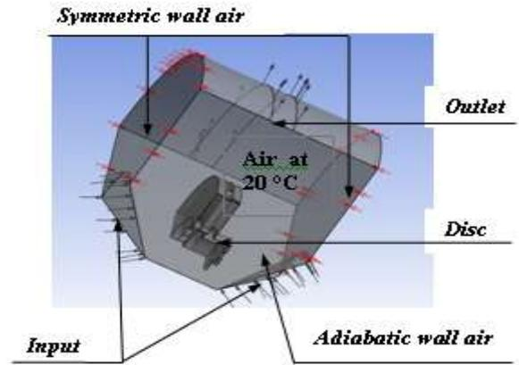
Fig.4 Brake disc CFD model
