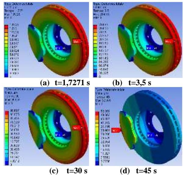
Fig13. Total distortion distribution
