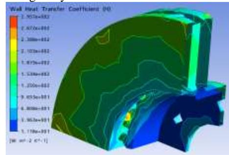
Fig.5 Distribution of heat transfer coefficient on a ventilated disc in the stationary case (FG 15).
