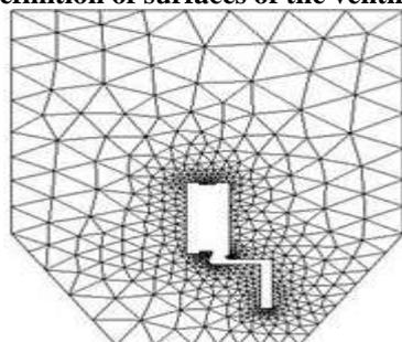
Fig.3. Irregular mesh in the wall
