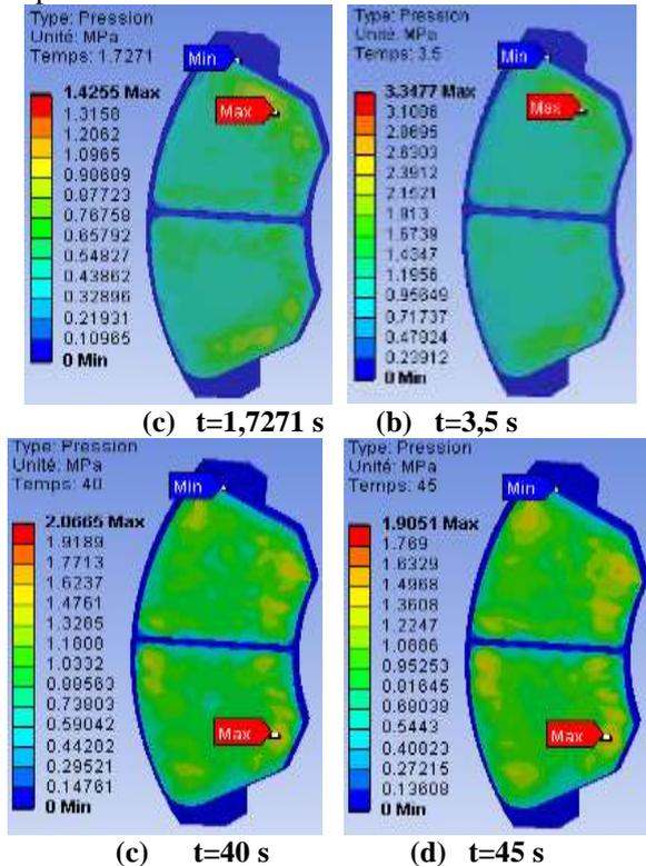
Fig.15. Contact pressure distribution in the inner pad
