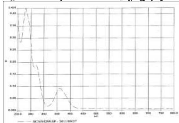
Figure 10: Uv spectrum of Cu^{2+}:(C_{17}H_{12}N_3O_2 S Cu)
