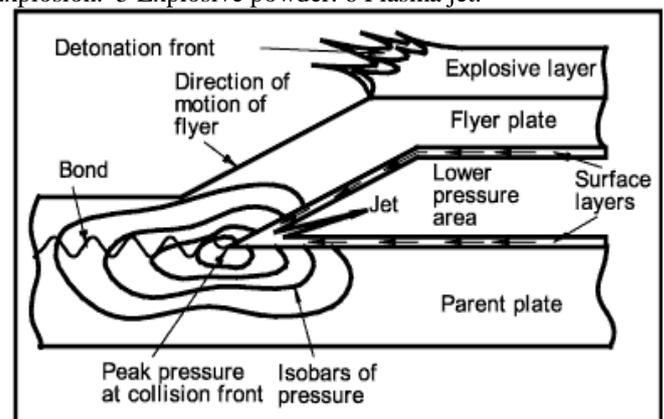
Fig.1. Dynamic situation at the collision front showing the jetting mechanism
