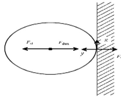
**Fig.3 Force balance of a vapor bubble at lift-off**
