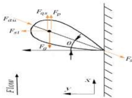
**Fig.2 Forces applied on a bubble in its nucleation site**
