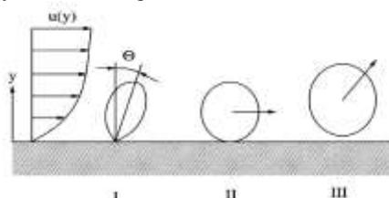
Fig. 1 Three stages of a vapor bubble departing from the heater surface
