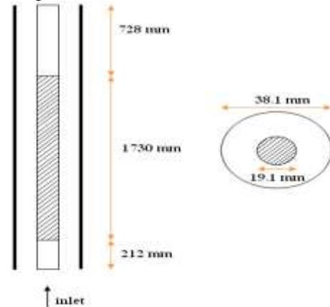
**Fig.4 Test section of BWR facility**
