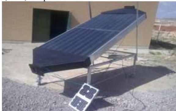
Figure 1. Flat plate surface solar collector
