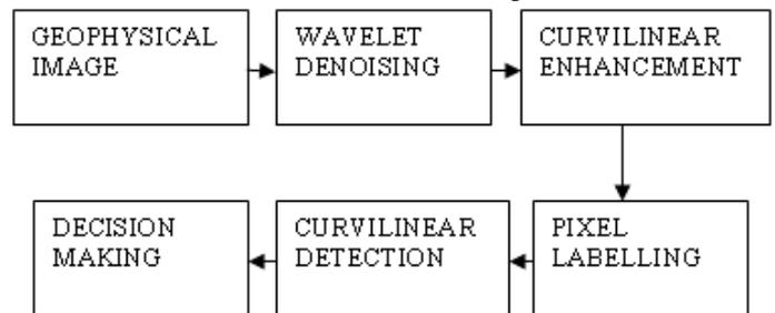
Fig.2 Scheme of the proposed system architecture
