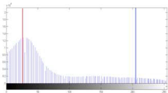
**Figure 5. The image histogram of enhance image and final cluster centers.**
