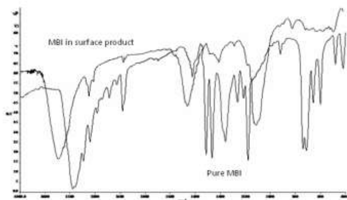
Fig. VIII FT-IR spectra of MBI both as pure form and in metal surface product
