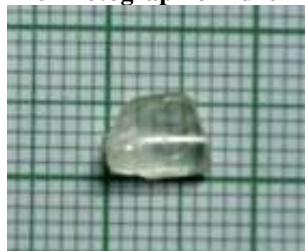
Fig. 1(b) The Photograph of L-Arginine doped ZTS crystal
