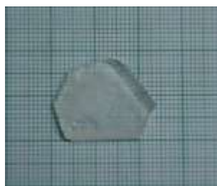
Fig. 1(a) The Photograph of Pure ZTS crystal
