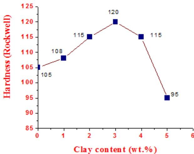
**Figure 3 Hardness test results of epoxy/polyester blend as a function of nanoclay**
