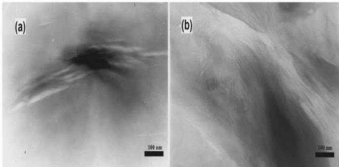
**Figure 2 TEM analyses of epoxy/polyester blend as a function of nanoclay at 3 wt% clay.**
