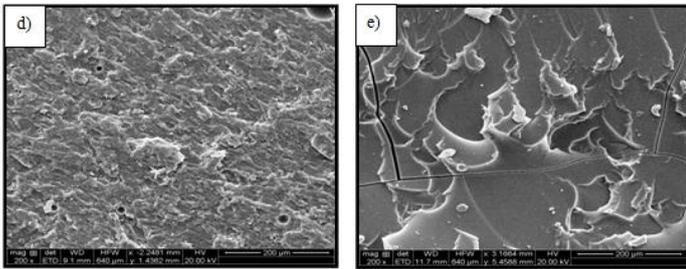
**Figure 1 SEM analysis of epoxy/polyester blend as a function of nanoclay at (a) 0 wt% clay (b) 1 wt% clay (c) 2 wt% clay (d) 3 wt% clay (e) 5 wt% clay.**
