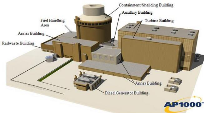
Fig.1 AP1000 PWR Schematic Building Design
