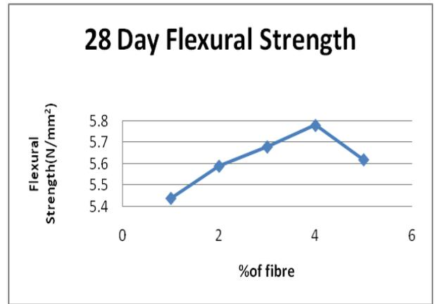
3) Graph Flexural strength of concrete and % of fibre
