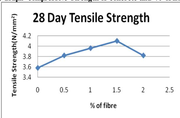
2) Graph Tensile strength of concrete and % of fibre
