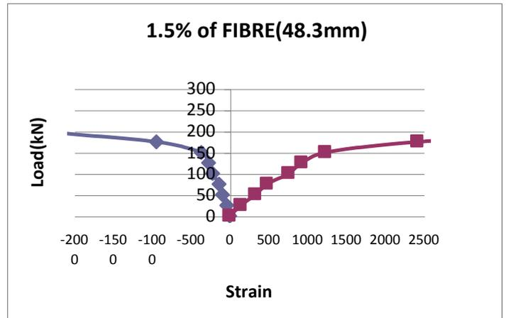
5) Graph Load (Y axis) vs. linear (-)and lateral strain(+)
