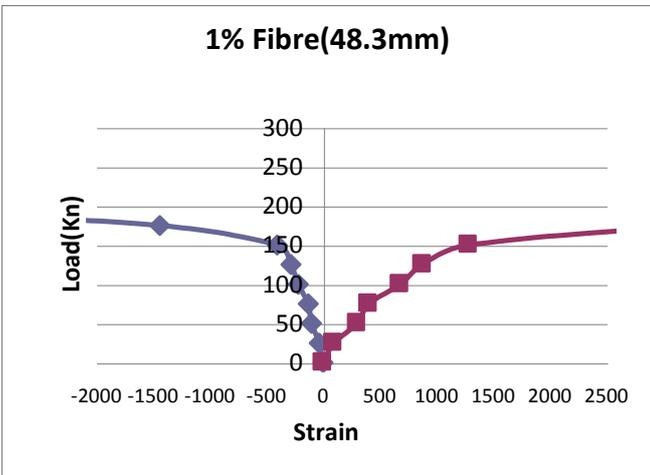
5) Graph Load (Y axis) vs. linear (-)and lateral strain(+)
