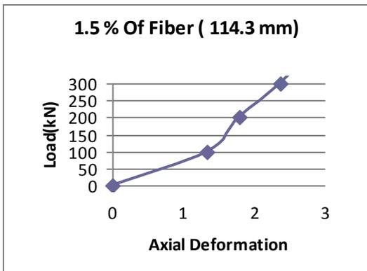
6) Load Versus Axial Deformation
