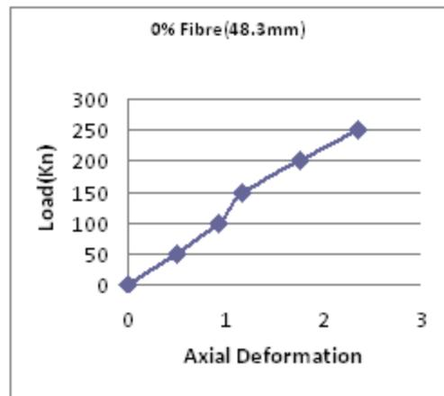
6) Load Versus Axial Deformation
