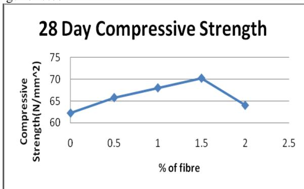
1) Graph compressive strength of concrete and % of fibre
