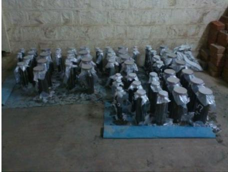
Fig.2. Specimens of concrete filled tubes
