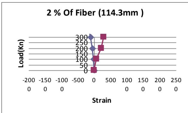
5) Graph Load (Y axis) vs. linear(-)and lateral strain(+)
