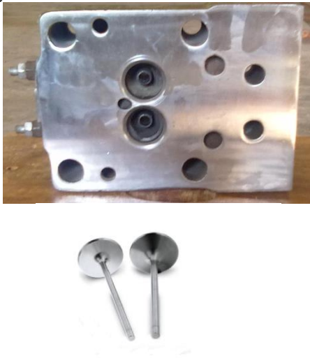
Fig 2: PSZ coated cylinder head and valves
