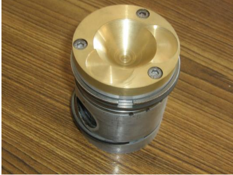
Fig.1: An air-gap insulated piston with brass insert
