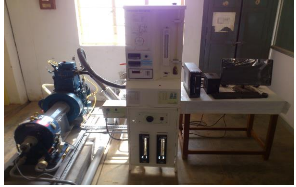
Fig. 3. Experimental set up of Insulated Engine Test Rig
