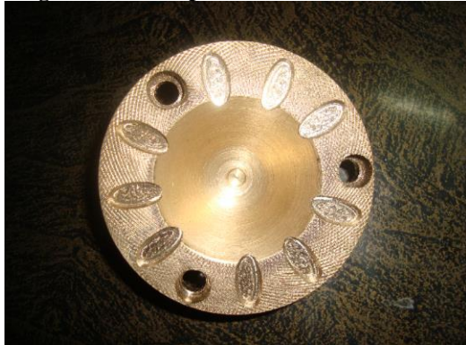
Fig: 7 Photo Graphic View of Brass Crown Piston With 9 grooves
