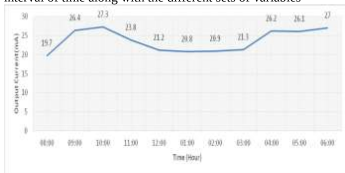
Fig 4. The output current of the electricity generated using geo-thermal energy
