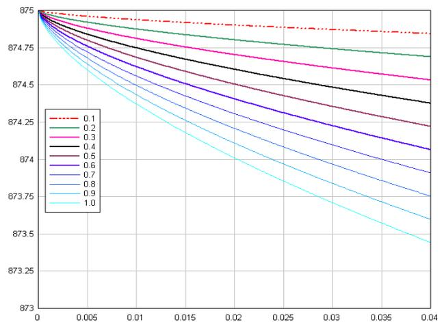
Figure.(4) Temperature distribution for Rectangular fin profile versus emissivity
