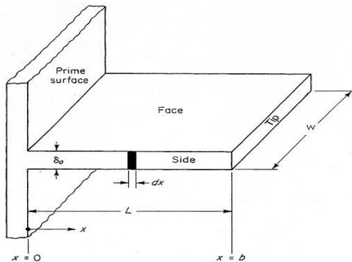
Figure.(3) Terminology and coordinate system for a radiating longitudinal fin of rectangular profile
