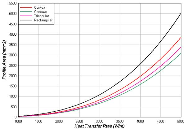
Figure.(1) Profile area for different types of Longitudinal fins
