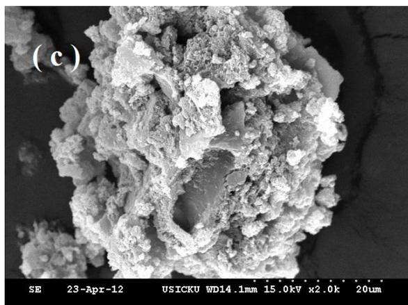
**Fig.2. SEM micrographs of (a) pure PANI, (b) [Co(meal)(H<sub>2</sub>O)<sub>2</sub>Cl<sub>2</sub>] complex, and (c) composite of [Co(meal)(H<sub>2</sub>O)<sub>2</sub>Cl<sub>2</sub>] complex with PANI**
