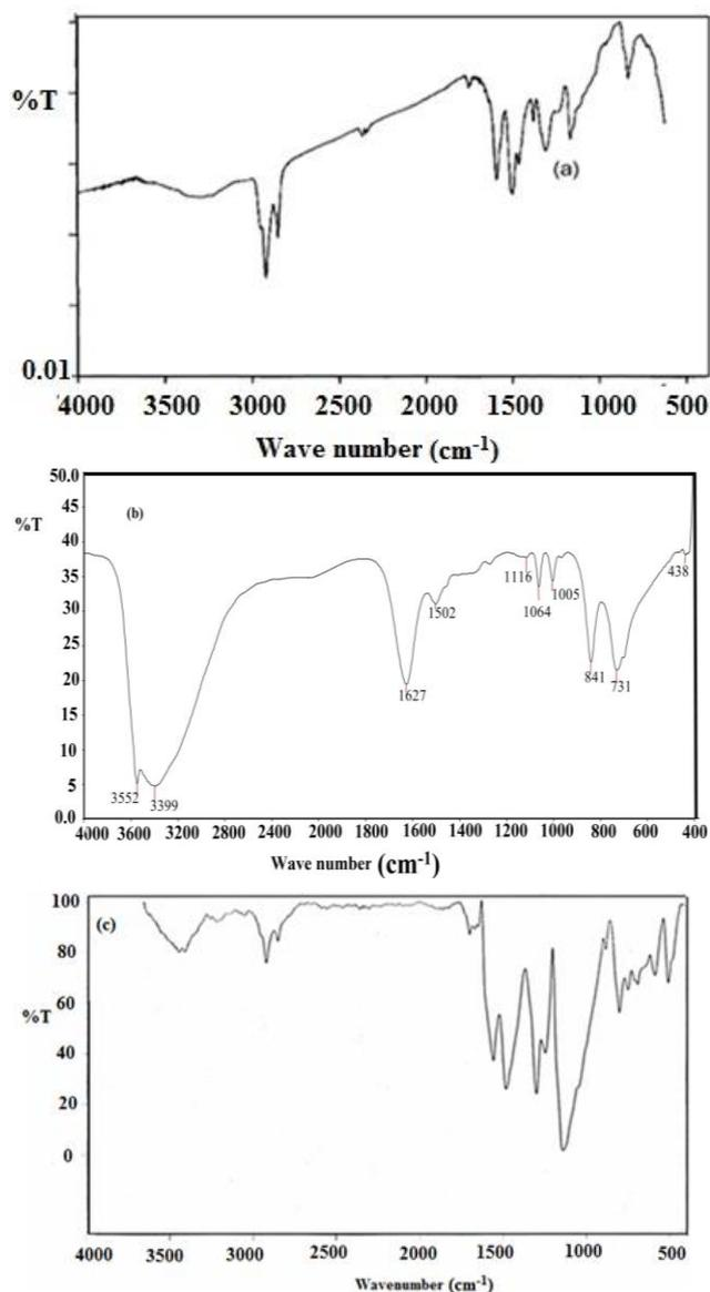
Fig.1. FTIR of (a) PANI, (b)  $[\text{Co}(\text{mea})(\text{H}_2\text{O})_2\text{Cl}_2]$  complex, and (c) composite of  $[\text{Co}(\text{mea})(\text{H}_2\text{O})_2\text{Cl}_2]$  complex with PANI
