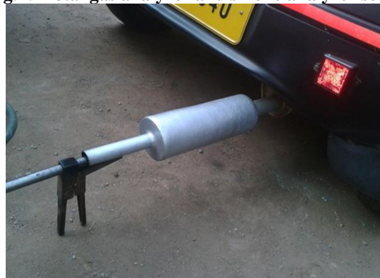
Fig.16 Experimental arrangement of the fabricated scrubber for testing
