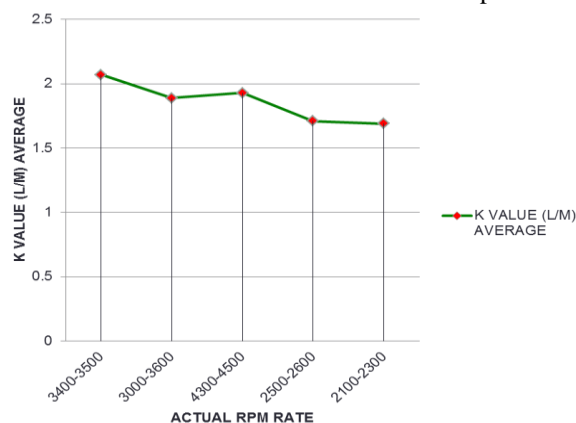
Fig.21 Light absorbing coefficient vs. rpm rates
