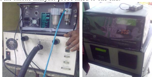
Fig.15 Total gas analyzer and smoke analyzer setup
