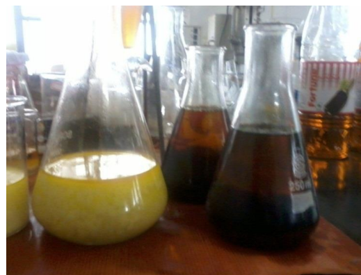
Fig. 3 Double Layers of Glycerol and Biodiesel – Removed fatty acids
