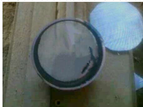
Fig.13 Ring sections of scrubber with wire mesh before fabrication
