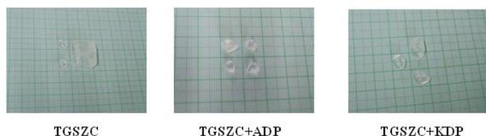
**Fig. 1 Grown crystals of pure and ADP-, KDP- (0.2 mol) doped TGSZC.**
