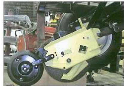
Fig. 12 Truax Rangeland Planter Boot installed on the planter
