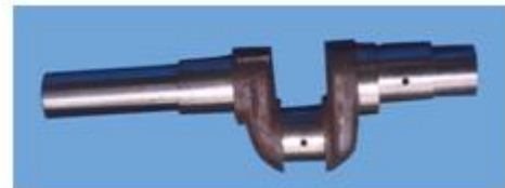
Fig.13 ADI Crankshaft for 5 HP single cylinder agriculture pump engine
