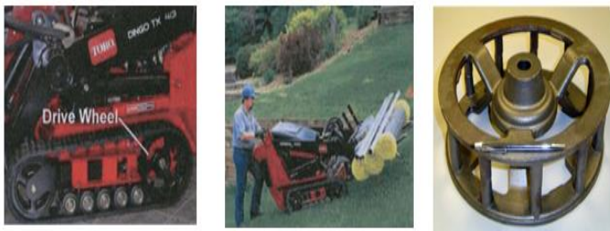
Fig.16. a) Toro Dingo TX drive system, b) Toro Dingo TX c)The one-piece ADI main drive wheel replaced an 82-piece steel welded and assembled component (Courtesy of Toro and Smith Foundry)
