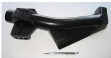
Fig. 11a A seed boot constructed of welded steel
