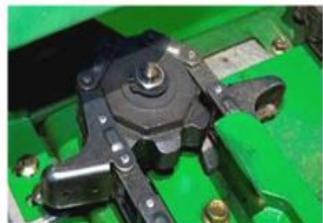
Fig. 20- This ADI adjuster sprocket is a durable alternative to steel
