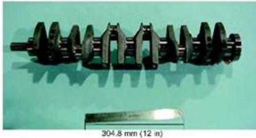
Fig. 10 ADI Crankshaft for TVR sports car
