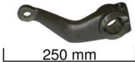
Fig. 15 Small ADI actuating lever for a European agricultural application
