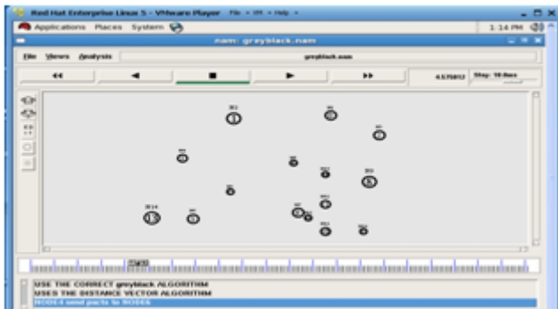
Fig 10: Implementing Distance vector algorithm for new routing table
