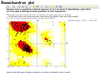
it's to visualize dihedral angles  $\phi$  against  $\psi$  of amino acid residues in protein structure. it shows the possible conformations of  $\phi$  and  $\psi$  angles for a polypeptide.all the residues were found with in allowed region
