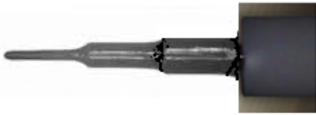
Figure 3. Electrode with 16 \mu\text{m} circular end shape Electrolyte concentrations
