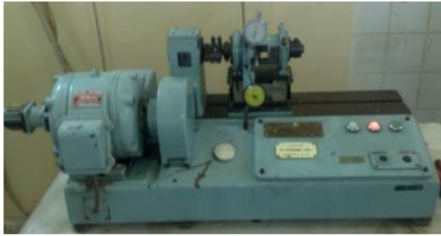
Figure (2-2) AVERY Fatigue Testing Machine Type 7305
