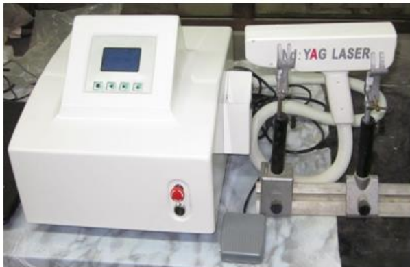
Figure (2-3) ND: YAG laser system
