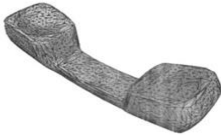
Fig.4 Polyhedral mesh representation (.stl file) of a part
