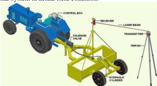
Fig.3 Schematic view of Laser controlled land leveling system
