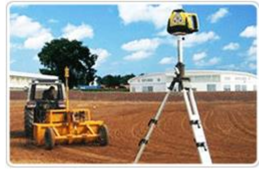
Fig.4 Laser controlled land leveling system in actual field The application and development of laser controlled land leveling System in Agriculture
