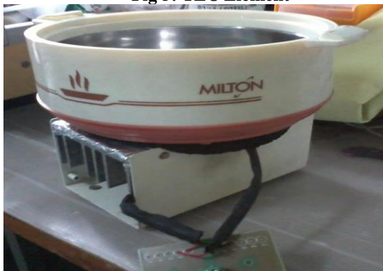
Fig 6: Cold storage before insulation
