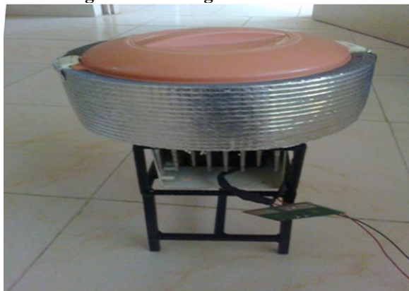
Fig 7: Cold Storage after insulation
