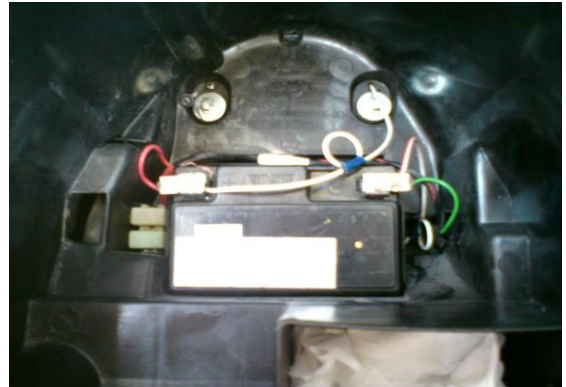
Figure 5: MBS electrical connection from motorcycle battery (power supply in transfer magnetic flux to MBS system)
