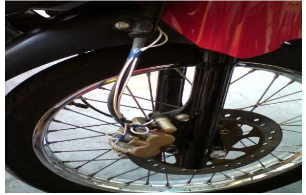
Figure 4 : MBS prototype installation on motorcycle brake disc
