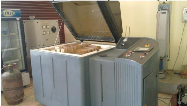
**Figure 1. Arrangement of sandwich specimens in salt fog chamber**
