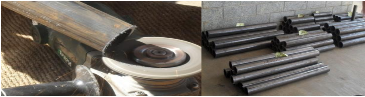
Fig 3. Cutting & preparation of Specimen to required Length
