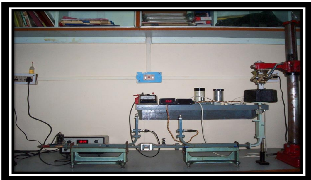
Fig : Microwave X- band set-up for dielectric measurements.
