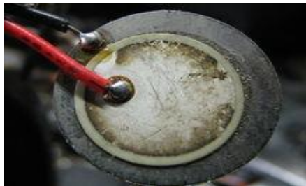
Fig.5: Metal disk with piezo-electric disk attached
