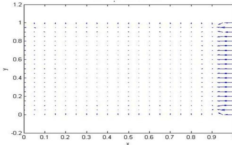
Figure 4(b): Velocity vector plot at the plane  $y = 0.9$  for  $Re = 2000$
