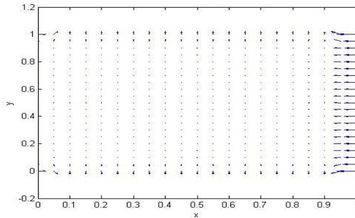
Figure 3(b): Velocity vector plot at the plane  $y = 0.5$  for  $Re = 2000$
