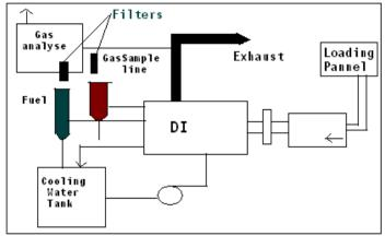
Except for the change in injection pressure and timing, there were no changes made in the engine. Injection pressure was varied from 180 – 340 bars. A standard fuel nozzle tester was used to characterize the spray. A Single Phase AC alternator was coupled to the engine main shaft and a resistance coils / light bulbs were used to load the engine. The fuel flow rate / consumption was directly measured by taking fuel level drop in a metering jar and corresponding time set the injector pressure.
