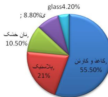
Figure 1. Physical analysis of dry waste collected by the waste bank station zone 11 December 2012
