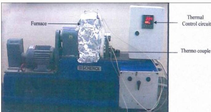
**Fig. 2 b. the fatigue-creep testing machine with furnace**
