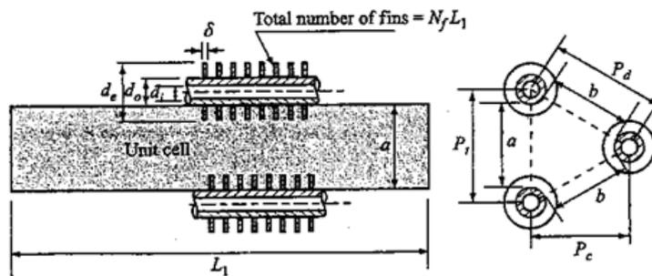
**Figure 3. Unit cell of a staggered finned-tube arrangement**
