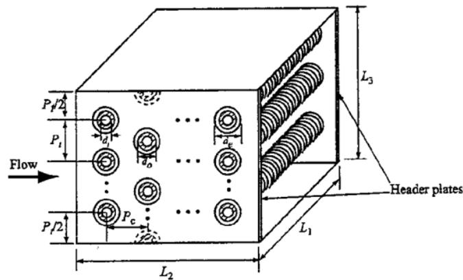
**Figure 2. Circular finned-tube heat exchanger**
