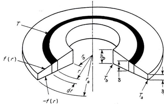
Figure 4. Coordinate system for a radiating radial fin of trapezoidal profile
