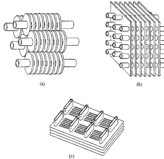
**Figure 1. Finned-tube heat exchanger (a) Circular finned-tube type.(b) Plate finned-tube type. (c) Louvered plate-fin flat-tube type**
