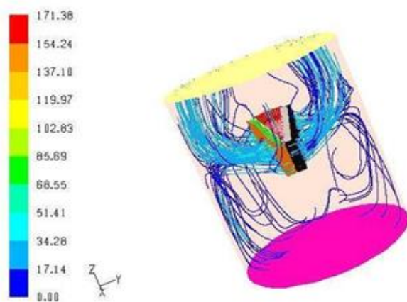
Figure 9. Contours of velocity magnitude streamlines for pure vapour feed
