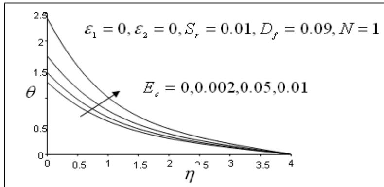
Figure 10: Variation of  $\theta$  for different  $E_c$  parameter for  $N = 1$ (aiding buoyancy)
