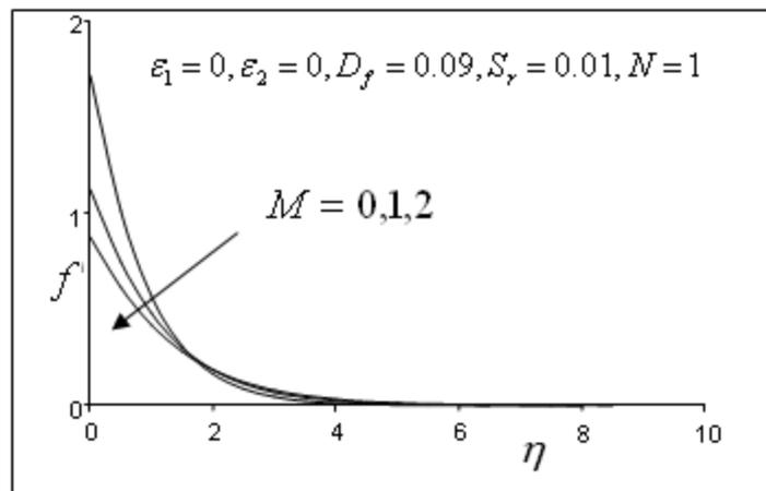
Figure 2: Velocity profiles for different magnetic parameter for N=1 (aiding buoyancy)
