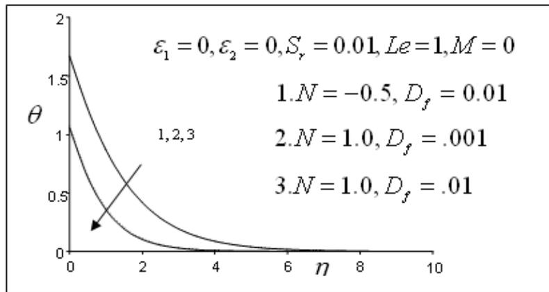
Figure 9: Variation of temperature both in aiding and opposing buoyancy
