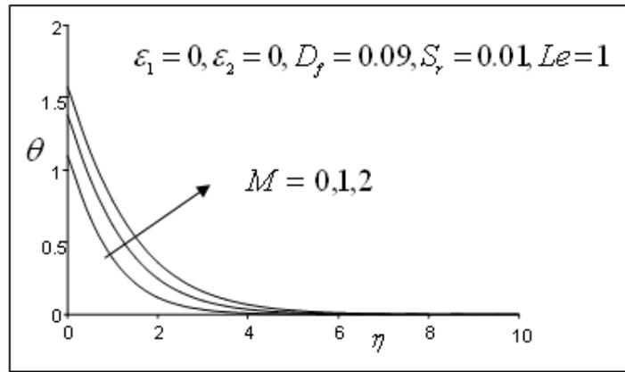
Figure 4: Temperature profiles for different magnetic parameter for N=1 (aiding buoyancy)
