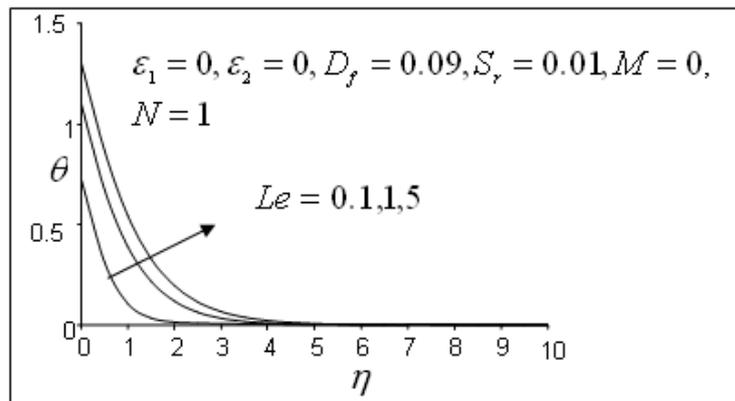
Figure 3: Temperature profiles for N=1 (aiding buoyancy)
