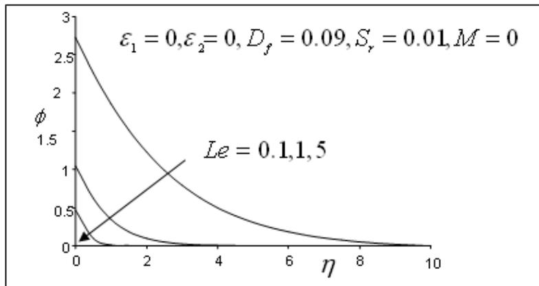
Figure 14: Concentration profile for  $N=1$ (aiding buoyancy)
