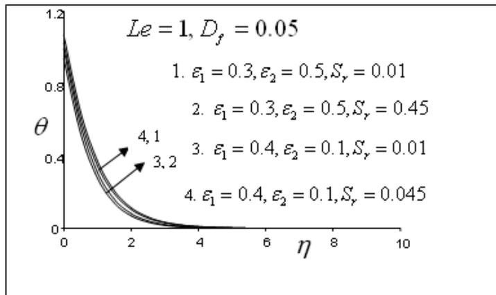
Figure 5: Temperature profiles for N=1 (aiding buoyancy)
