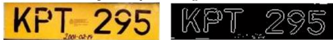
Fig. 3: Selected sample plate used as a filter before and after edge detection
