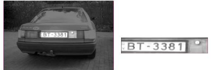
Fig. 6: Best candidate localization and selection respectively using sample plate as a filter
