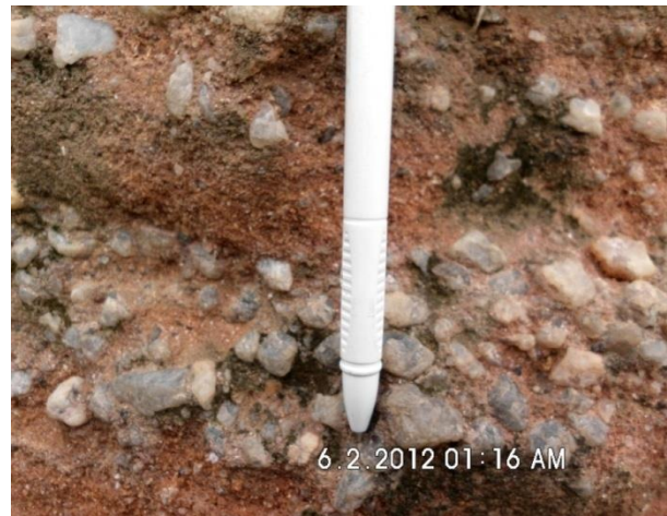
Figure 3: Conglomeratic feldspathic sandstone (cyclic deposit at Ori Ohin)
