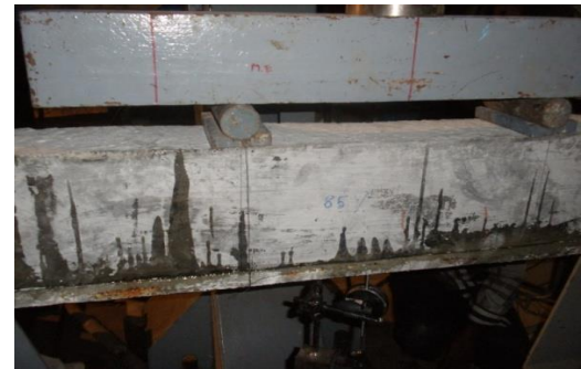
Fig 2. Beam strengthened on loading frame
