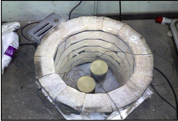
Figure 1. High temperature electric furnace with specimens
