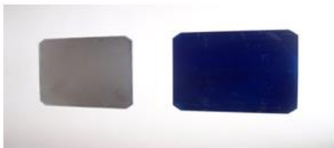
Fig 2.a: Photograph of Non-AR coated and AR Coated Silicon wafer
