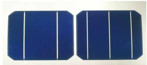
Fig 3.a: Front side pattern comparison – 2 Busbar vs 3 Busbar
