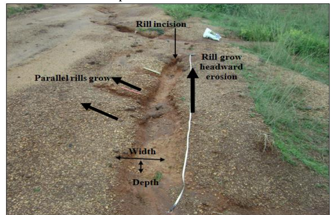
Figure 5. Rills Development during rainy season at Rangamati (July, 2012, width 12 cm and 6 cm depth)
