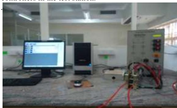
Fig 1. Fuel cell test station
