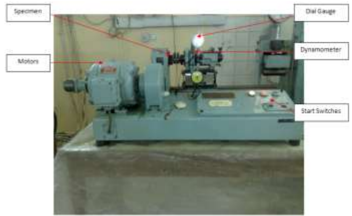
Fig 3. Fatigue Test Device
