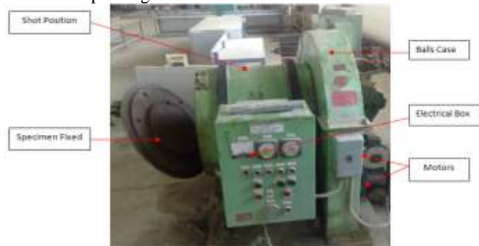
Fig 2. Shot Peening Device
