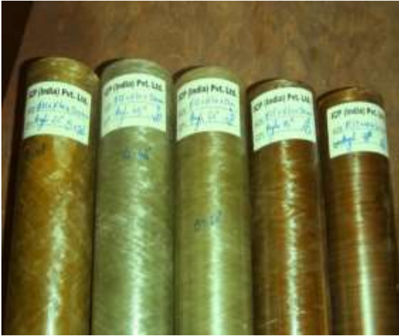
Figure 1. Photo graph of the GFRP Tubes Table 2. Process parameters and their levels
