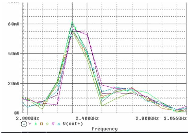
Figure 8: VCO output spectrums for different value of temperature
