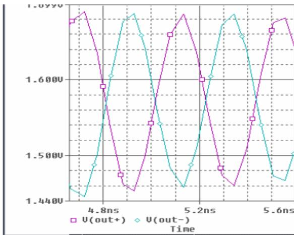
Figure 7. Output waveform of LC oscillator
