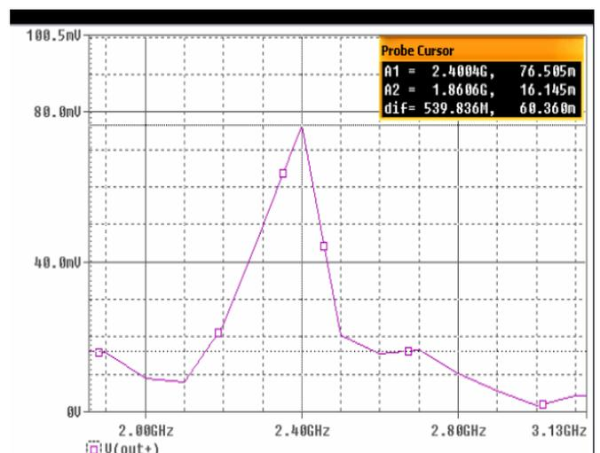
**Figure 6. Frequency spectrum of LC oscillator**
