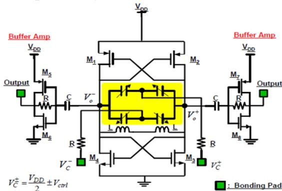
**Figure 5: Schematic of a typical VCO with differential outputs.**
